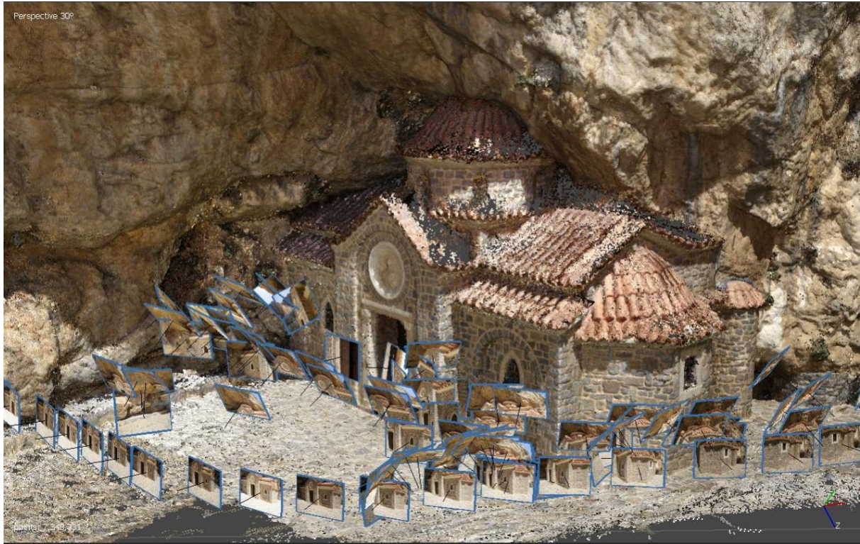
Figure 1 – 3D model of Church Agios Nikolaos, Crete - screen capture of SFM software Agisoft Metashape . The blue squares represent the visual content and approximated spatial location of images captured.
